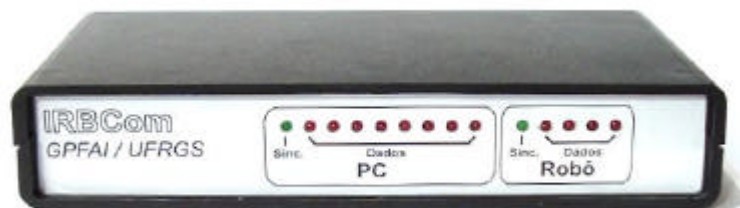
Figura 3.7 – Painel frontal do módulo IRBCom
