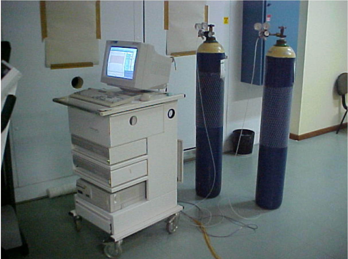
Figura 3 - Ergoespirômetro de circuito aberto e analisador de gases marca MedGraphics Cardiorespiratory Diagnostic Systems , modelo CPX/D da Medical Graphics Corporation .
