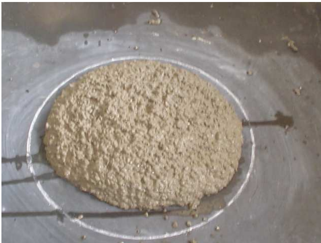
Figura 9: ensaios de slump flow test com o slum flow T 50cm test
