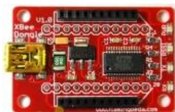
Figura 3.6: XBee Dongle.
