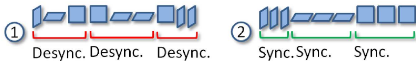
Figure 5.6: (1) Quadtree cell list presenting arbitrary alignment sequences. (2) Quadtree cell list presenting alignment-based grouping sequences. Alignment-based cell grouping improves performance by reducing divergence during kernel executions.
