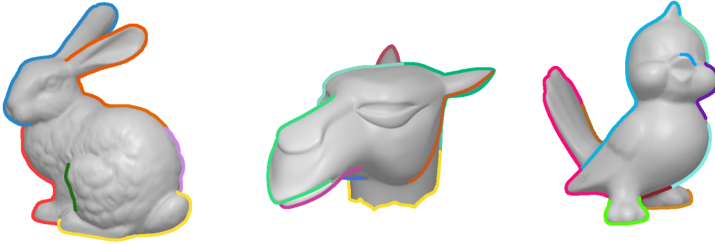
Figure 4.2: Silhouette Detection. Results of silhouette detection algorithm applied to Stanford Bunny, Camel and Tweety.
