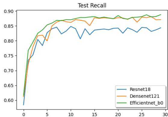
Figure 5.3 – Evolution of the recall on the test set across 30 training epochs for the three candidate architectures.
