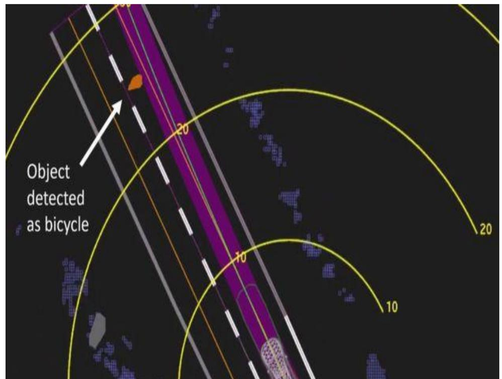
*Image copyrightNTSBImage captionThe US National Transportation Safety Board (NTSB) mapped the incident - yellow rings show metres ahead of the vehicle, orange lines centre of mapped travel and purple area the car's path*
