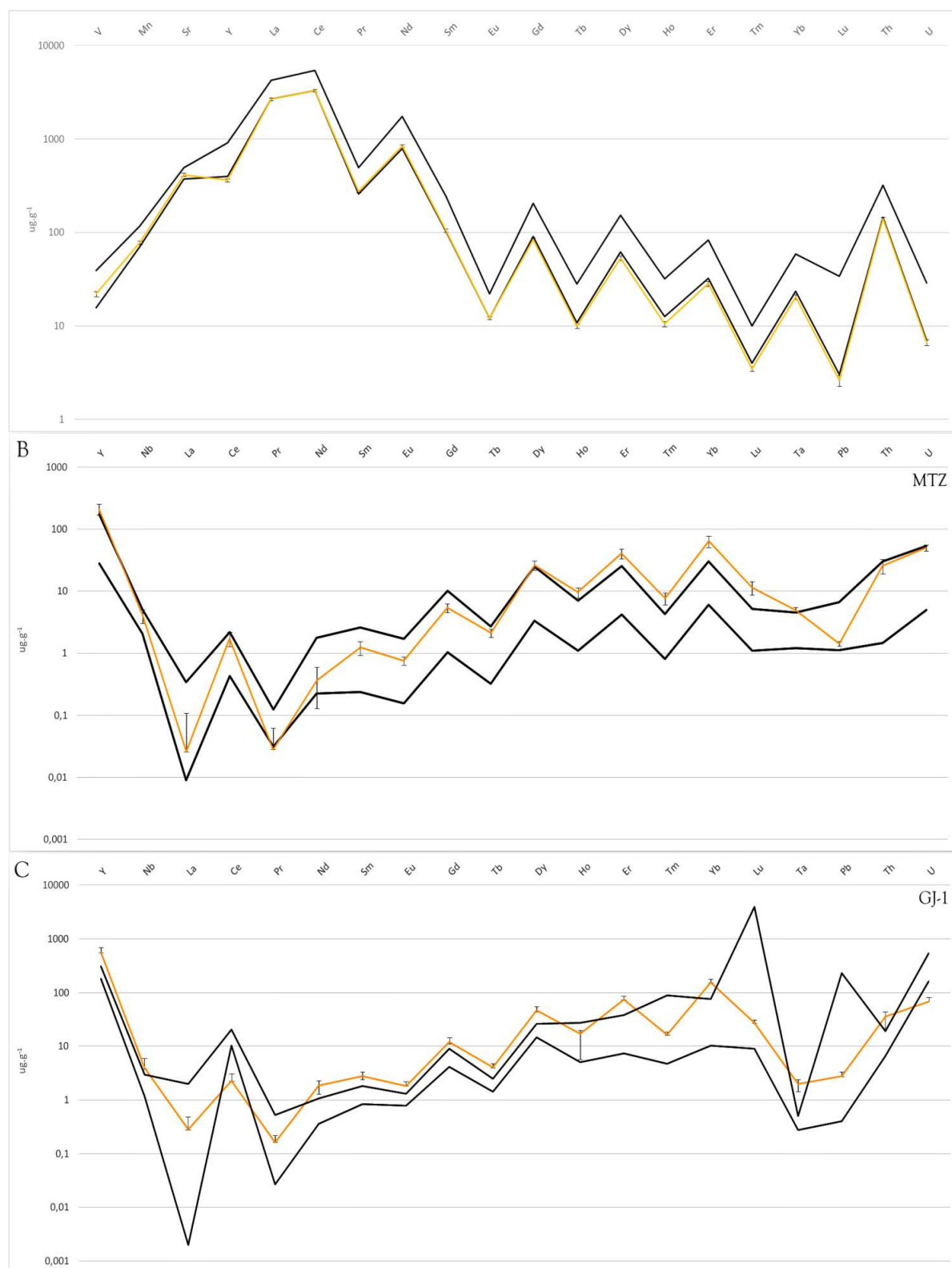
Figure 2: LA-ICP-MS trace element concentrations ( \text{mg.g}^{-1} ) for mineral phases obtained in this study (orange lines), compared to maximum and minimum values reported in literature (black lines). Error bars are two standard deviations ( 2\sigma ) of the mean value. (A) TE concentrations for Durango Apatite. (B) TE concentrations for Mud Tank Zircon. (C) TE concentrations for GJ-1 Zircon.
