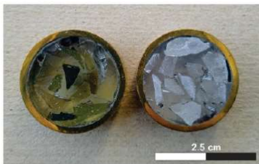
Figure 1 Glass beads produced in this study; sodium borate + rock powders (left) and only sodium borate, which was as necessary to control blank measurement and possible contamination from the flux (right).
