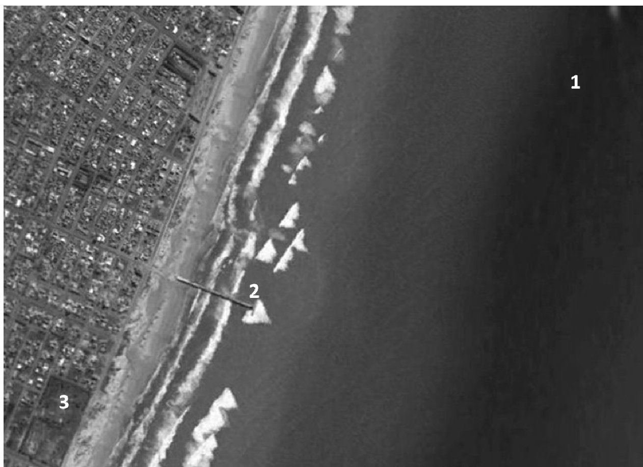
Figure 3. Position of Tramandaí beach on the State's northern coast. The Google Earth® image shows the three points of data collection: currents on the fishing platform (2), wind on the land-based meteorological station (3); the site of the wave recorder is also shown (1).
