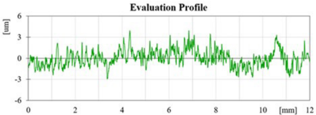
Figure 11. Roughness profile of the machined surface of sample 20.
