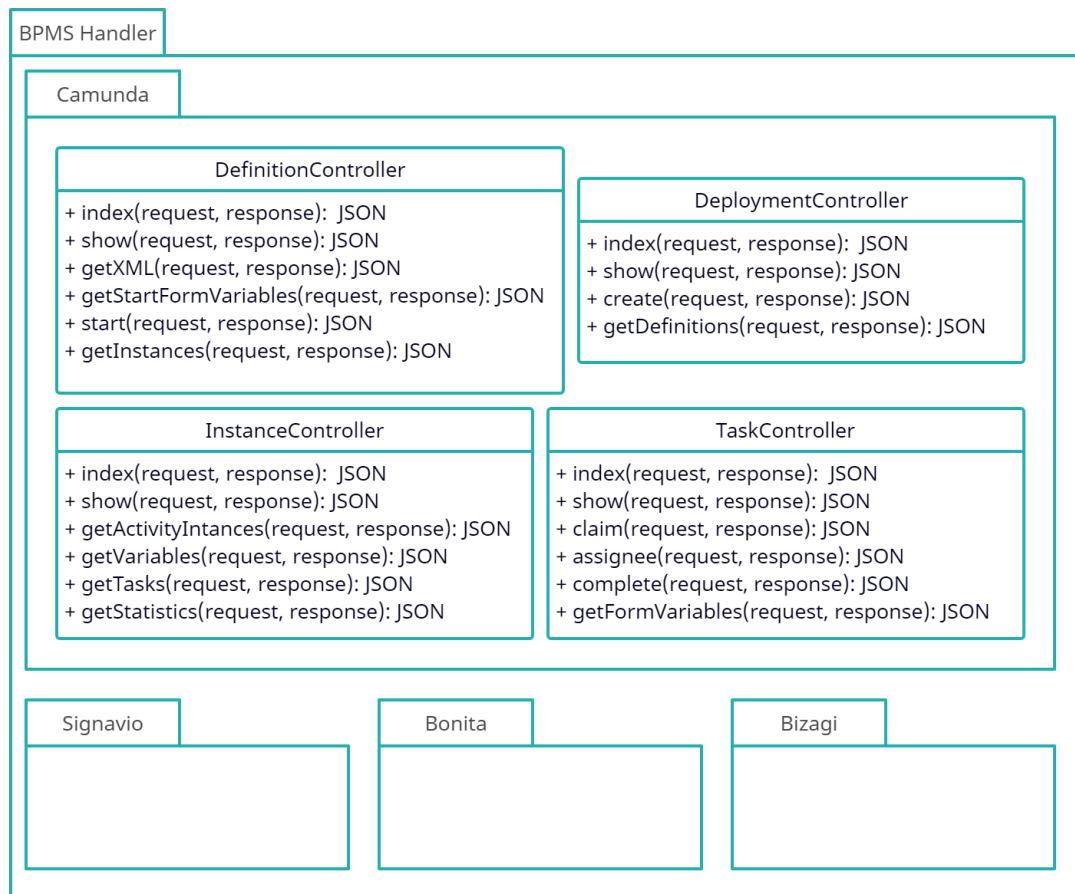
Figure 4.7: BPMS Handler class diagram
