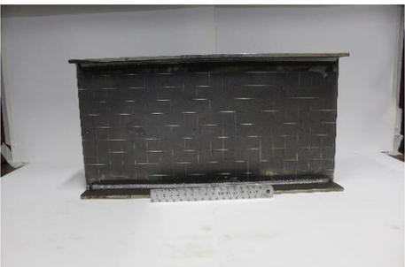
A photograph of a welded joint between two metal plates. The joint is a simple butt weld. A ruler is placed below the joint for scale. |
