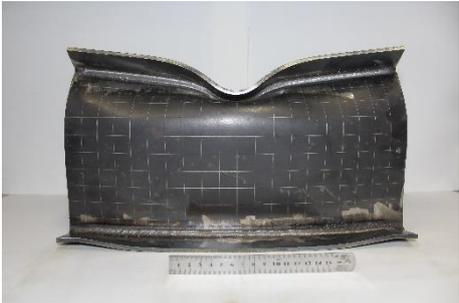
A photograph of the same welded joint after a test. The joint has deformed significantly, with the metal plates curving downwards and outwards. A ruler is placed below for scale.   |
