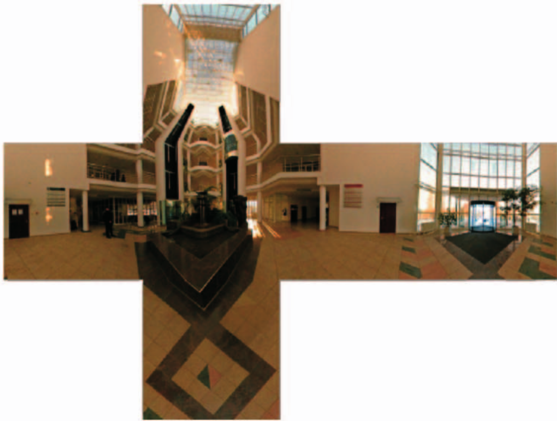
Figure 2.3 – Image projected to a cube (cube map). Extracted from Wan, Wong and Leung (2007)
