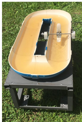
Fig. 11. Low-cost, homemade raceway pond reactor. Source: Author.
