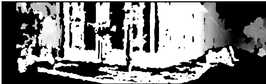
Figure 3.6: Depth estimated from stereo camera. Frame from the KITTI odometry dataset.
