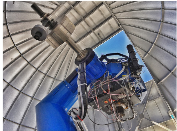
Figure 4. T80S and its wide-field camera.
