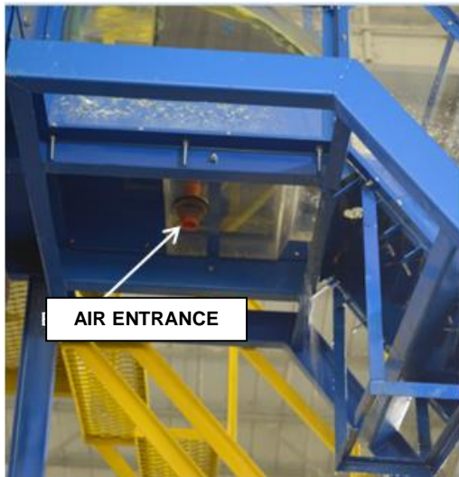
Figure 1. Lateral view of the air chamber of the air induction system.
