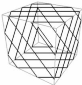
Figure 1. Texture-based visualization uses parallel planes orthogonal to the viewing direction to sample the volume.
