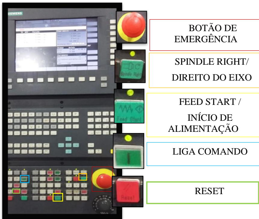
Painel de controle
