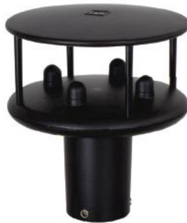
Figure 3.27 – Gill WindSonic ultrasonic anemometer
