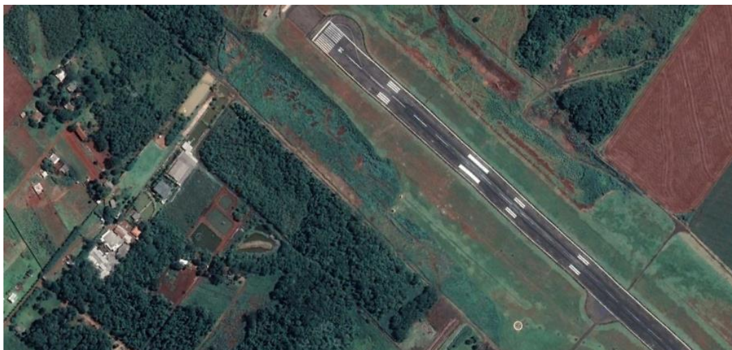
Figure 3.25 – Satellite image of SBFi – Foz do Iguaçu, PR, showing razing of vegetation immediately adjacent to the runway (Dated 29/01/2019).
