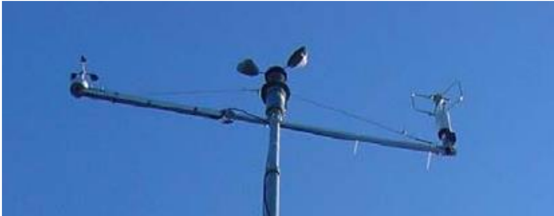
Figure 3.26 – Vaisala WAA151 cup anemometer (left), Synchrotac 706 cup anemometer (middle), and RM Young Model 8100 3D ultrasonic anemometer (Gorman, 2004).
