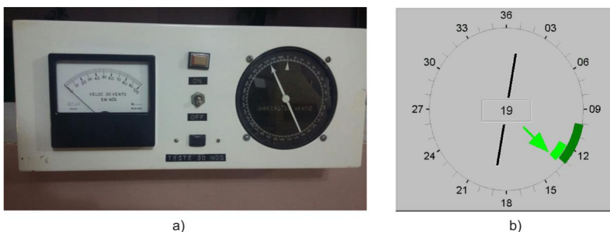
Figure 3.3 – Wind speed and direction readings by a) analogue and b) digital processes.
