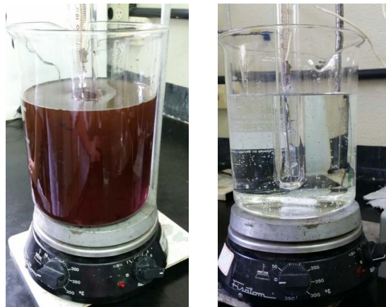
Figure 9. Aspect of the synthetic effluent containing the 4 dyes before and after the application of the photocatalytic treatment with ZnO (2.5 g L -1 in aqueous solution with 8% ethyl alcohol), UV irradiation, temperature-controlled system at 30 °C and pH 10.
