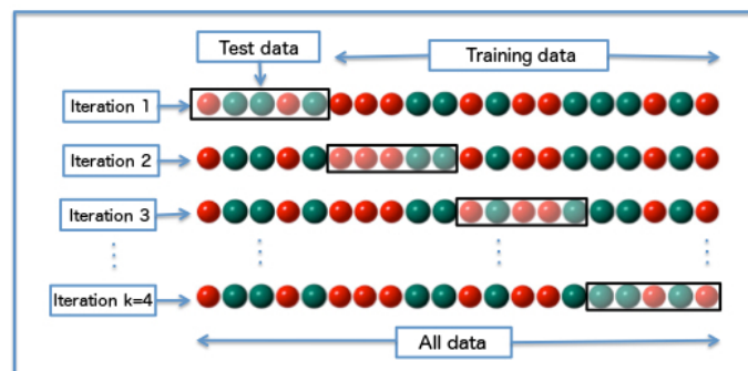
Figure 2.16: Diagram of a k -fold Cross Validation, with k = 4 .
