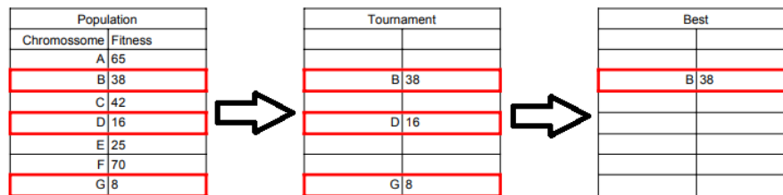
Figure 2.6: Tournament Selection example, with size = 3 and p = 1 .
