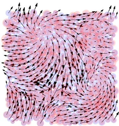
FIG. 6. Example of soft mode with \omega \approx 0.078 for \bar{\alpha} = 1 and \Delta = 10^{-2} . Blue disks indicate the initial particle radii, red disks the new radii induced by motion along that mode. Arrows represent the displacements \delta \vec{r}_i of the particles multiplied by 4 for visualization.
