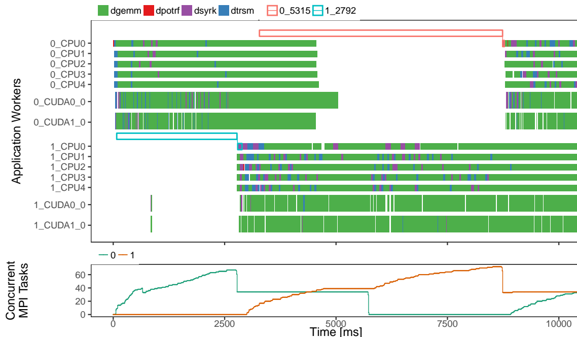
Figure 6.9: The first 10000ms of a StarPU-MPI multi-node execution of the Cholesky factorization with a matrix of 75 \times 75 tiles of 960 \times 960 using the DMDAS scheduler. The additional panel depicts Concurrent MPI operations which enables a correlation with long MPI transfers delaying tasks 0_5315 and 1_2792 .
