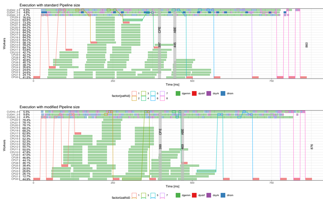
Figure 8.9: Comparison of a execution with the standard pipeline size (top) and the modified one (bottom).
