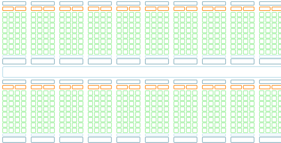
Figure 2.1: The layout of a hypothetical accelerator. Green boxes represent computing units (cores), orange ones the control system and blue ones the memory hierarchy.
