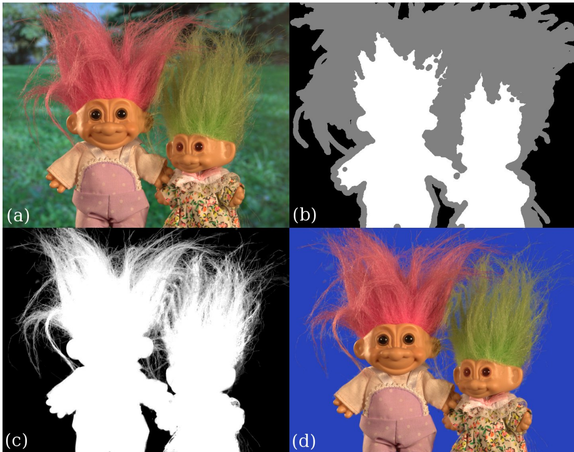
Figure 1.1: Example of alpha matte extraction and compositing using the proposed technique. (a) Image ( 800 \times 563 pixels) from the training dataset provided by (RHEMANN et al., 2009). (b) Trimap provided in the dataset, with 40% of unknown pixels (gray represents unknown regions, while black and white represent known background and foreground regions, respectively). (c) Alpha matte computed with the proposed technique in 0.043 seconds. (d) Composite of the extracted foreground on a new background.
