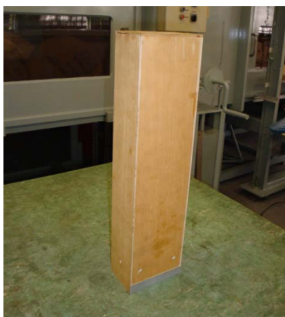
Figura 5.5 – Modelo do CAARC Standard Tall Building .
