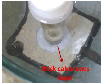
Figure 5.28: Photographs showing the specimen (with holiday) exposed to 60°C seawater after 17h showing the holiday covered by a visible deposit of calcareous matter, pH 9.2.
