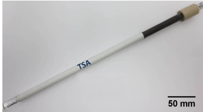
Figure 4.14: Glass rod TSA-coated previous to the exposure test in synthetic seawater.
