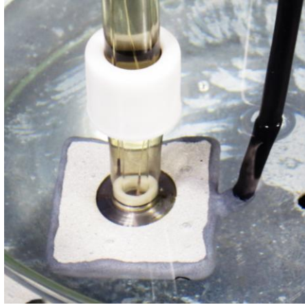
Figure 4.17: Photograph showing the specimen with 20% holiday exposed to the seawater showing the pH probe centred within the holiday.
