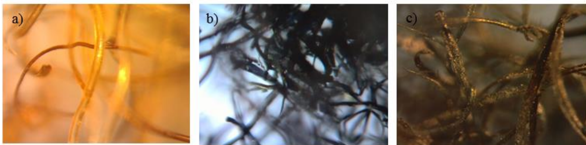
Fig. 3 Optical Microscopy of CHW (a) before adsorption; (b) after adsorption with AB-161 dye and (c) after adsorption with AB-210 dye.
