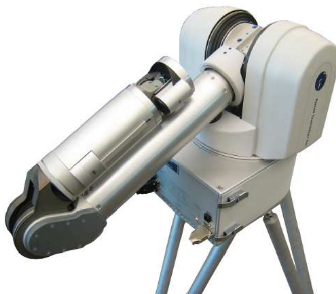
Figura 1: Manipulador Barrett WAM. (BARRETT TECHNOLOGY INC, 2015b)
