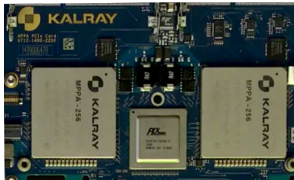
Figure 1: Two Kalray MPPA ® -256 processors in a board
