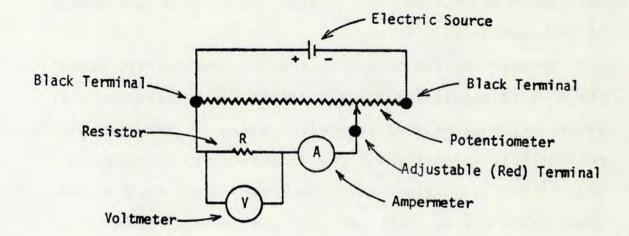
In this circuit, by varying the position of the adjustable terminal of the potentiometer one can vary the electric potential difference applied on the resistor R which can be measured by the voltmeter. With the ampermeter one can measure the corresponding electric current. However, in this circuit the ampermeter is actually indicating the current that flows through the resistor R plus the current that flows through the voltmeter. Another possibility would be to make the following connection:
