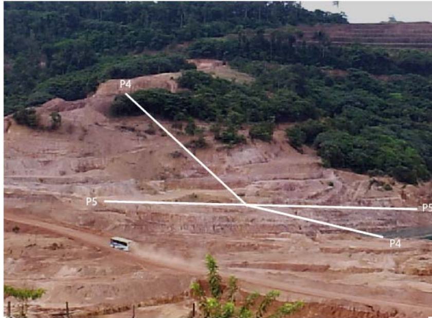
Figure 3. Photo with a field image of soil from border albite-enriched at the edge of the open pit with profile P4 and horizontal level P5. The number of samples increases from the bottom to the top in the P4 profile and from left to right in the P5 level.
