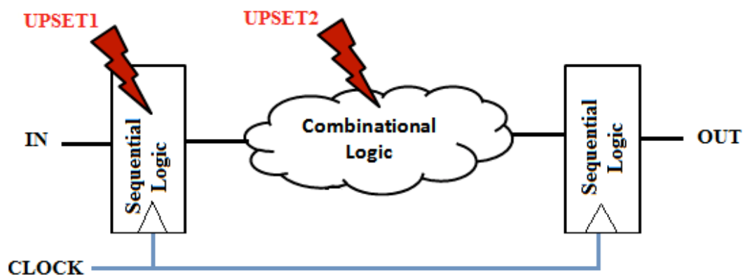
Figure 2.4: Upsets possibilities: combinational or sequential logic circuits. Adapted from (KASTENSMIDT et. al, 2006)
