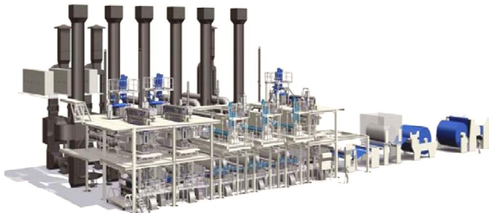
FIGURA 3 - ESQUEMA DE LINHA PRODUTIVA DE NÃOTECIDO SSS E SSMMS (REICOFIL, 2009)
