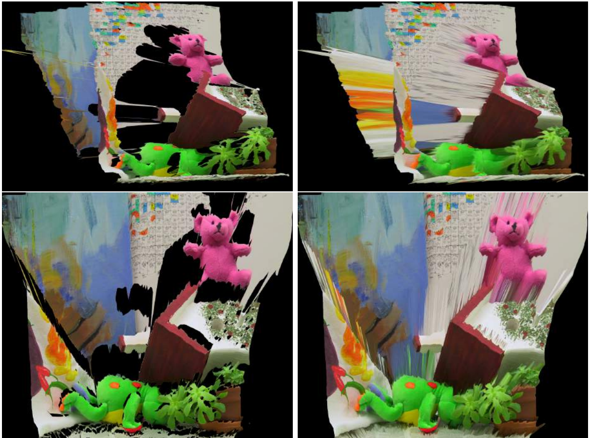
Figure 3.16 – 3D textured mesh for the Teddy dataset rendered using two different viewpoints for the synthetic camera (top and bottom). On the left column are the mesh rendered without orthogonal triangle, and on the right column are the meshes rendered with the orthogonal triangles.
