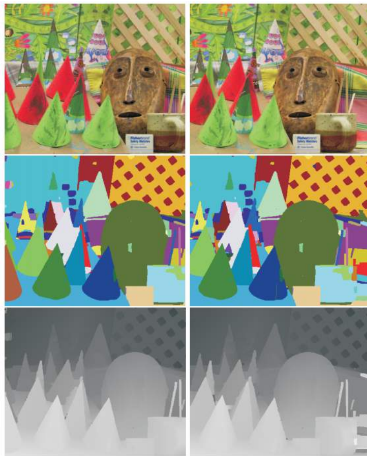
Figure 2.2 – Joint segmentation and disparity estimation results from Bleyer et al. (2011). On top row we can see the stereo images, in the middle row the obtained object segmentation and in the last row their respective disparity maps.
