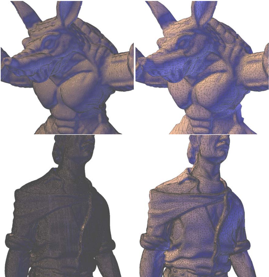
Figure 7.6: Armadillo and Laçador Results. Detail from Original Mesh and Saliency-guided Simplification to 5% of original resolution.
