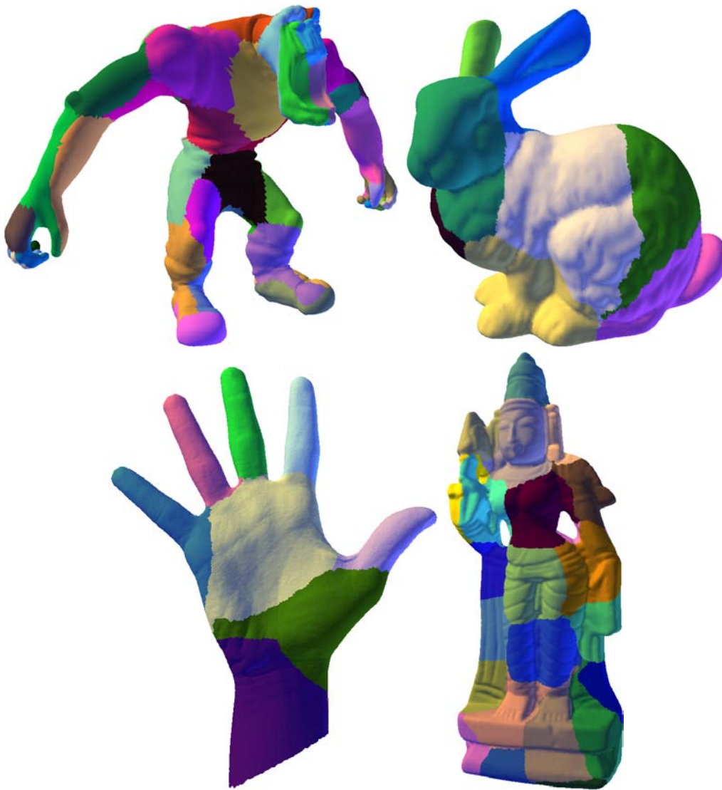
Figure 1.3: Mesh saliency is used to perform salient clustering which is suitable for view-dependent rendering. Segmentation results for the Grunt, Bunny, Hand and Goddess1 datasets.
