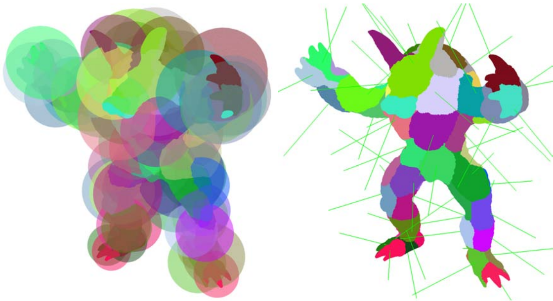
Figure 6.2: Cluster bounding spheres and mean normals.
