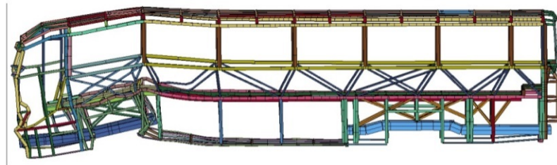
Figure 21 Deformed configuration for 8.89 m/s.
