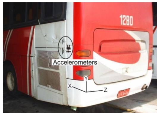
Figure 8 Location of accelerometers.
