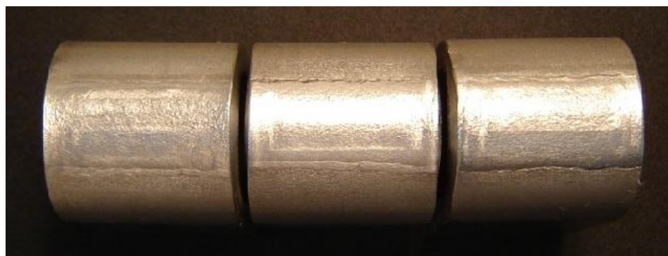
Figura 6.25 – Dobramento transversal de face.
