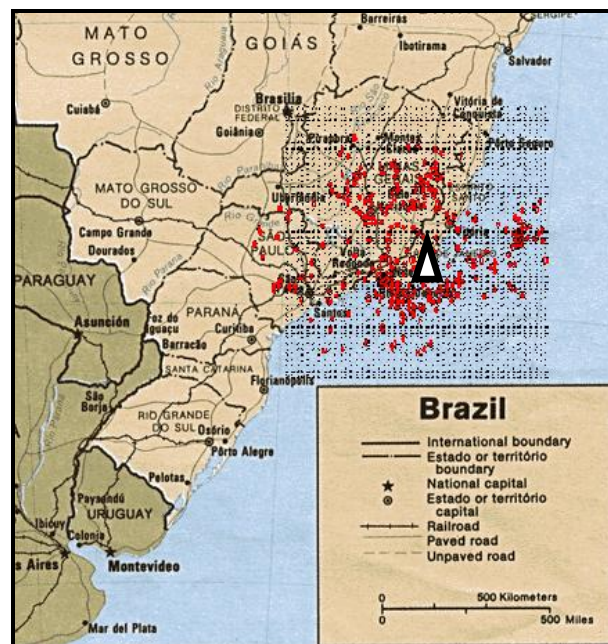
Figure 2: Distribution of Epicenters of Seismic Events ( M_w \geq 2 ) Occurred in the 50 Years Period between 1961 and 2011 within the Square Region Shown in South-Eastern Brazil. The Big Triangle at (23.08° S, 44.45° W) Shows the Site of the Angra dos Reis NPP (CNAAA)
