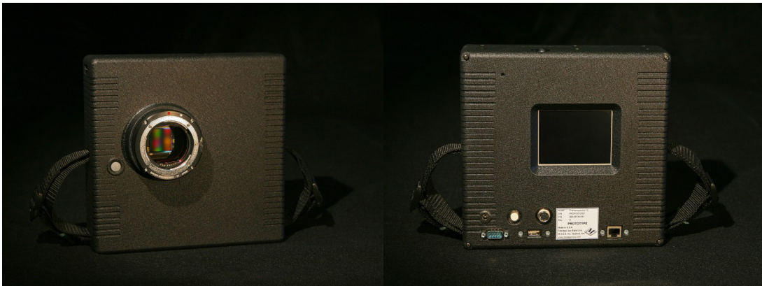
Figure 2.1: The Frankencamera (Camera 2.0) developed in Stanford University
