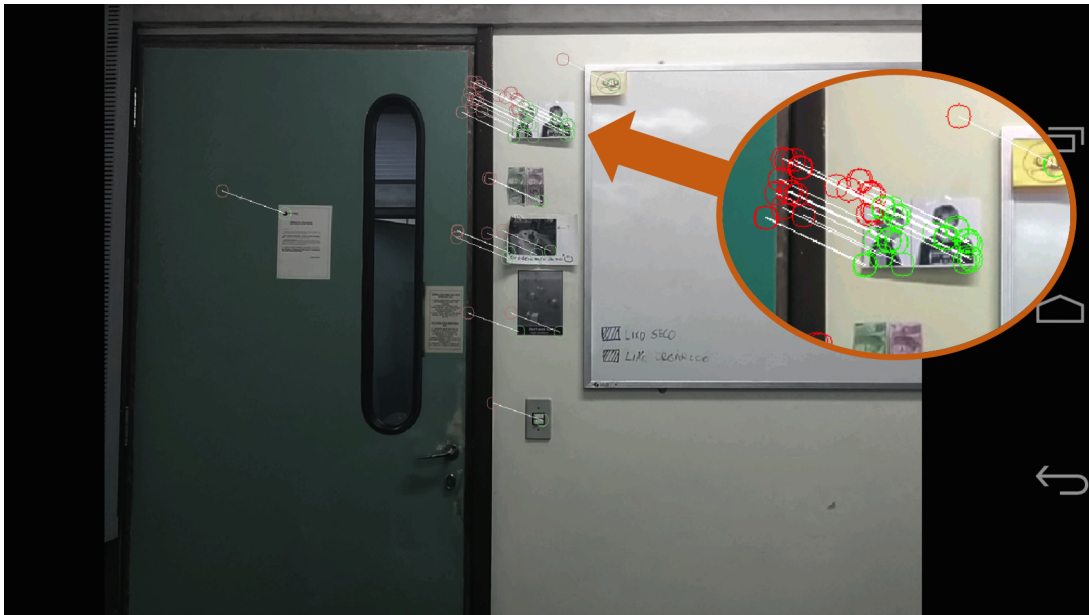
Figure 3.7: The matched keypoints. Red are the ones from the reference photograph and green, the ones from the current frame.
