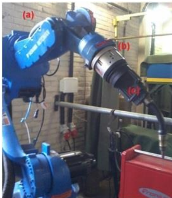
Figura 4.4 – (a) Robô Motoman MA1400, (b) Manipulador iCAT e (c) Tocha Robô WH.
