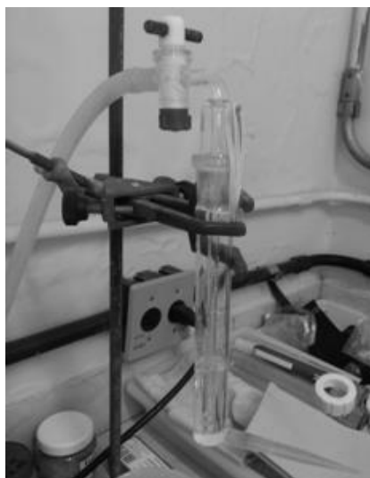
Figure 2. Device used for measuring the total gas volume generated in the bioreactors.
