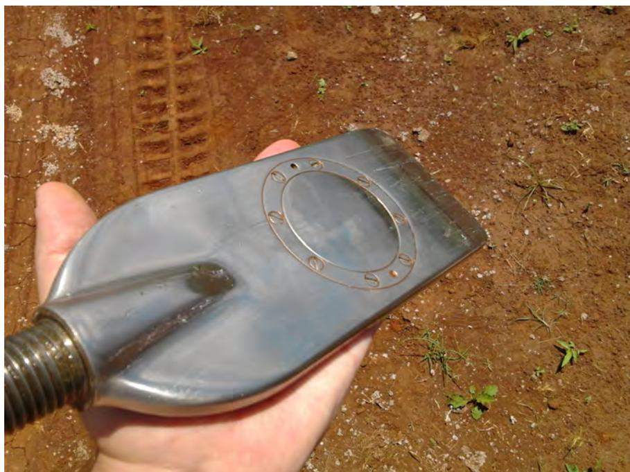
Figura 6.10 – Lâmina do *Flat Dilatometer Test* (DMT).
